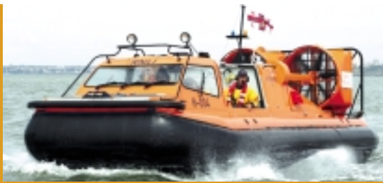
Griffon Hovercrafts use two TDI® 1.9 engines in the Type 470 craft they build for the RNLI.
